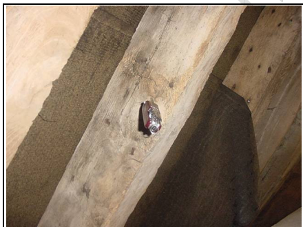
Knife test for softness
