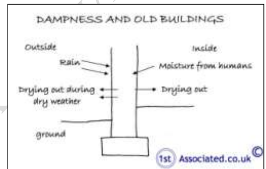
Dampness in old buildings
