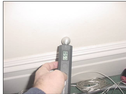
Damp readings with a Gann meter
