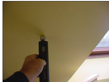
Damp readings with a Gann meter
